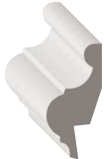
STOCK CODE 6PM (1522168) DIMENSIONS 1 1 / 16 " x 2" x 8-16' ADJUSTABLE 1/4" X 3/4" RABBET PIN
